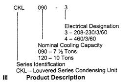
When matched with the appropriate airhandler(s) or evaporator coil(s) the CKL090/120 condenser complies with the rminimum efficiency equirements found in ASHRAE 90.1-1999. See the Goodman
